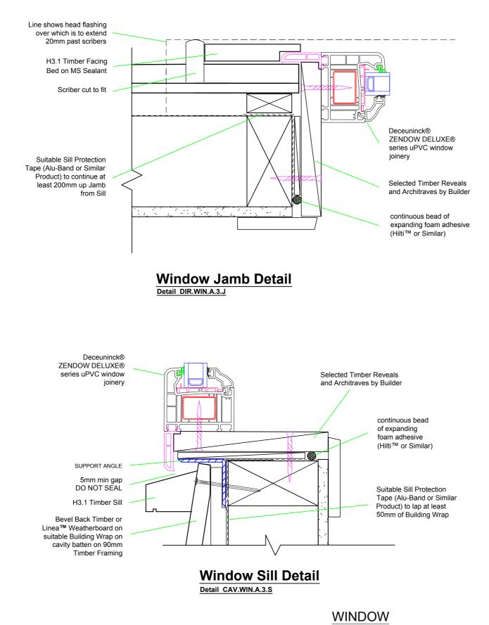
Bevel back weather boards on cavity batten with timber facings
