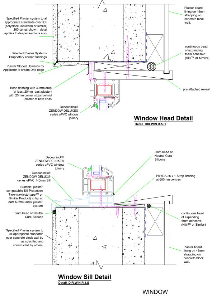
Concrete masonry block
