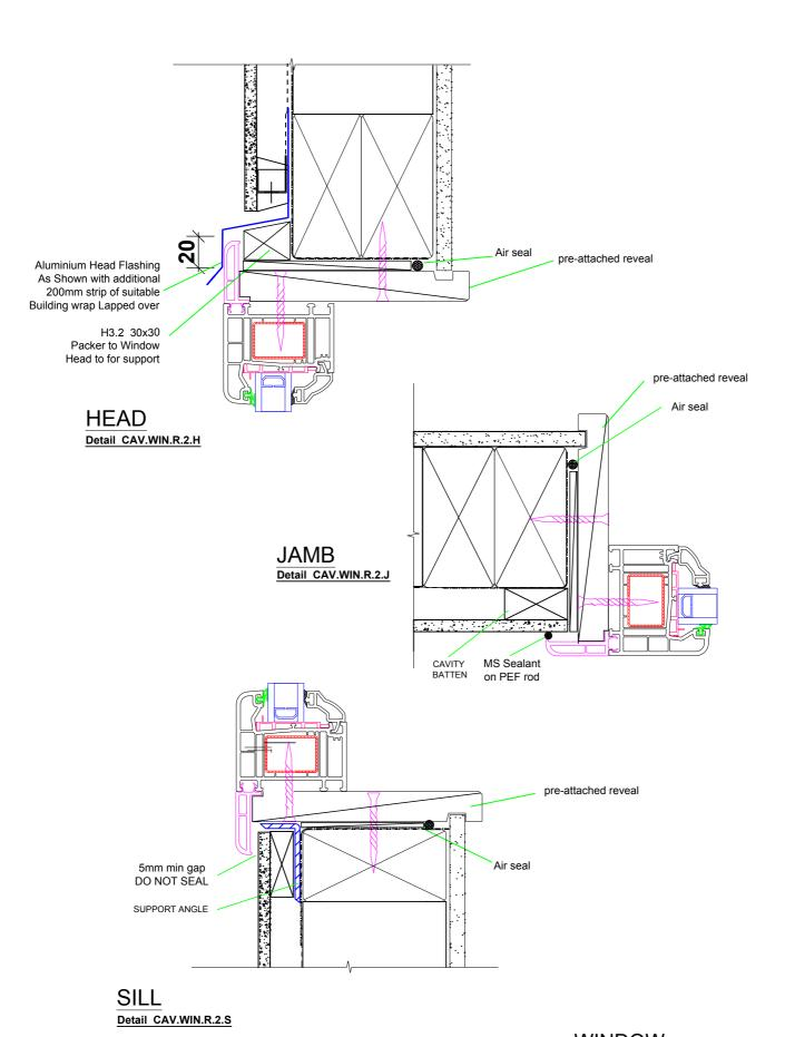
WINDOW Sheet Cladding on cavity
